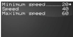
The "Speed" reading indicates the speed set, and varies in real time when the **↑** and **↓** keys are pressed. Any variation in speed is memorised as a parameter specific to the current product type.
