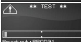
The Metal Detector requires an operational test to be carried out (see "Periodic test management" section below)
