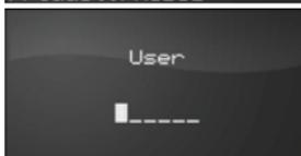
Programming access phase: the metal detector requires to type an user name, and possibly a password. The cursor position indicates where the next character will be typed.
